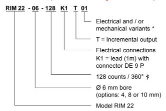
**Please note:** Standard magnetic actuators have an internal bore to accept shafts of 6 mm dia. Actuators with 4, 8 or 10 mm dia must be ordered **separately**, e.g. RBM-N08, for quantities up to 24 pieces. For larger quantities such actuators will become part of the standard item as per the order code, e.g. RAM 22 - **08** - 360 K1 W C01.
