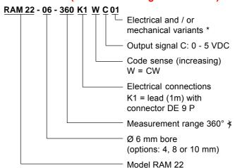
**Please note:** Standard magnetic actuators have an internal bore to accept shafts of 6 mm dia. Actuators with 4, 8 or 10 mm dia must be ordered **separately**, e.g. RBM-N08, for quantities up to 24 pieces. For larger quantities such actuators will become part of the standard item as per the order code, e.g. RAM 22 - **08** - 360 K1 W C01.
