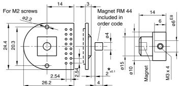
\* Distance between magnetic and sensor chip. Permissible coaxial tolerance ±0.1.
