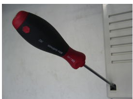
Remove the DCS550 Control Panel if present. Depress the locks to remove the cover
