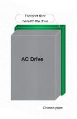
Drive mounted on an external footprint filter
